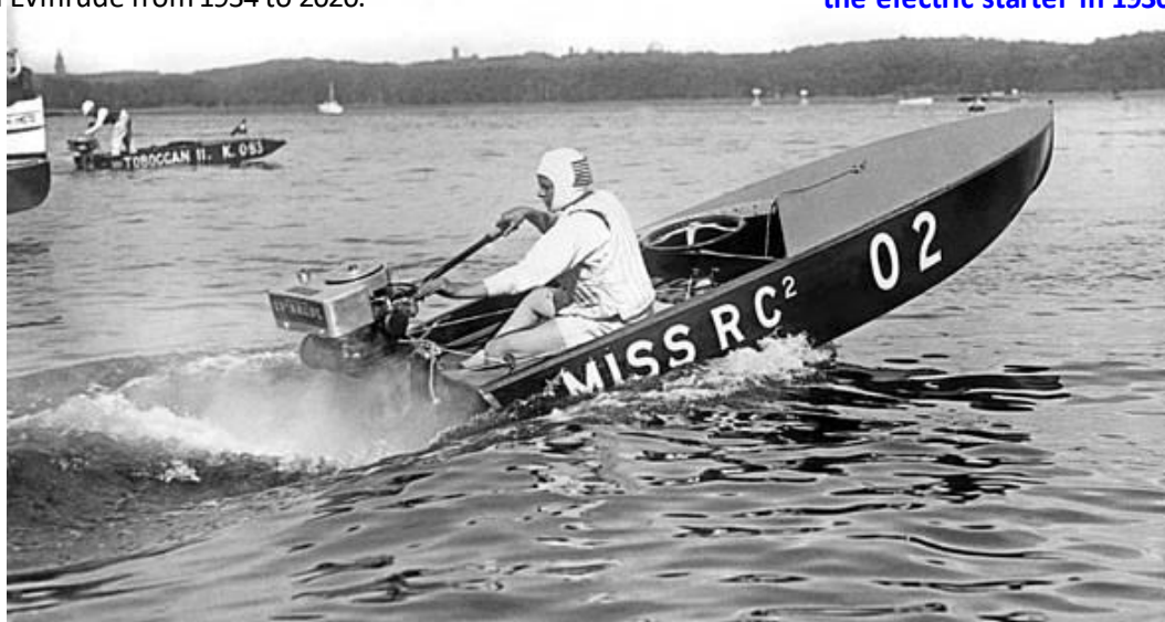
Boat racing victories became an important part of the Evinrude brand marketing program during the late 1920's & 1930's. Evinrude was the first to produce a factory racing motor with dual carburetors, the 1930 model 177 Speeditwin Racer.
