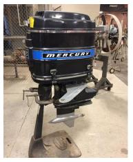
Mercury Twister 2 with Speedmaster racing gearfoot.
