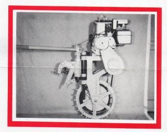
The POLAR MOTOR weighs approximately 97 lbs. and is powered by a 4 HP 4 cycle Briggs and Stratton air cooled engine. Five and 6 HP units are available on special order.
