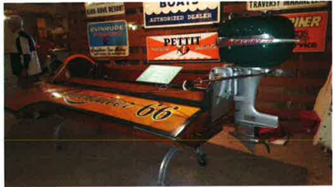
A/B Class Hydro, "Miss QuickSliver" built by Spike Burns. Motor is a Merc KG7H. From Ken Kirks Collection.
